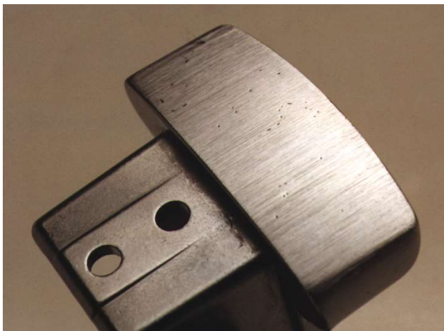
Figure 8. Shows porosity on a push bar end cap. The cluster is too dense for an A surface.
