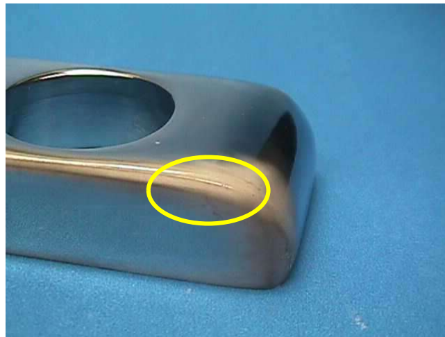
Figure 1. Chrome burn on a 334 cylinder control housing
