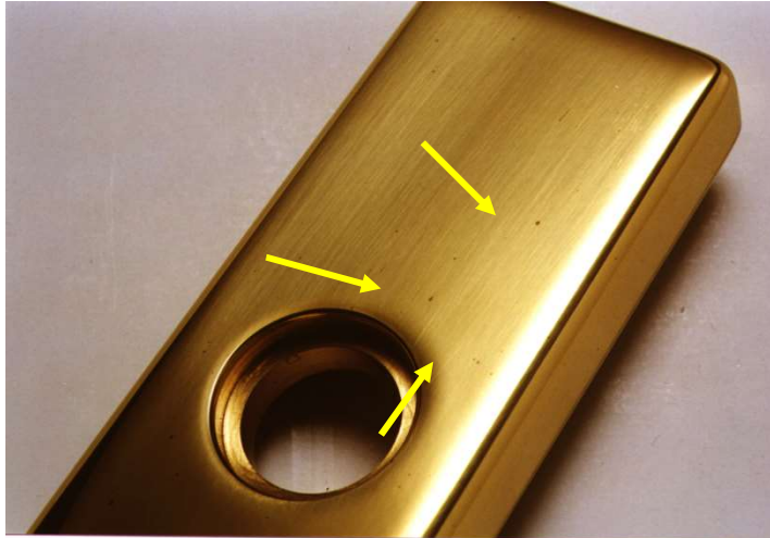
Figure 7. Polishing compound splattered on a 994 trimplate.
