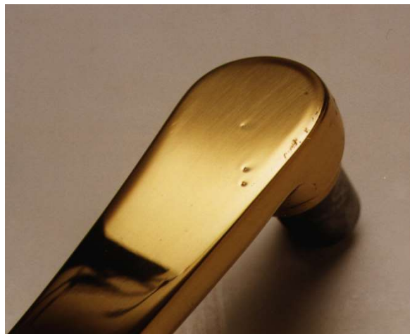
Figure 9. Shows pinholes on a lever. These holes are too large for an A surface.
